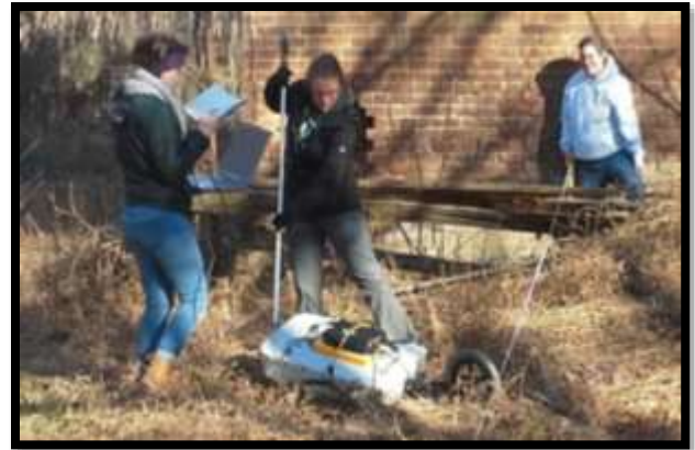
Dr. Sojka, Jessy Spencer & Allison Brooks surveying the Boydton property with GPR.
