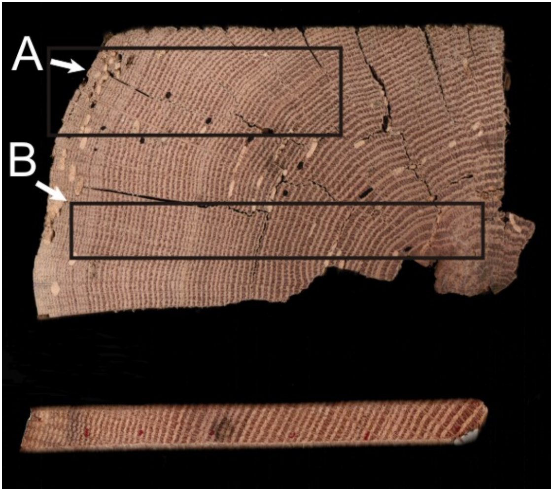
Figure 1. A cross-section of an oak timber with sapwood rings on the left-hand side (above). The boxes illustrate conversion methods resulting in A ) a precise felling date and B ) a terminus post quem or felled after date. Also pictured is a core showing complete sapwood (below).
